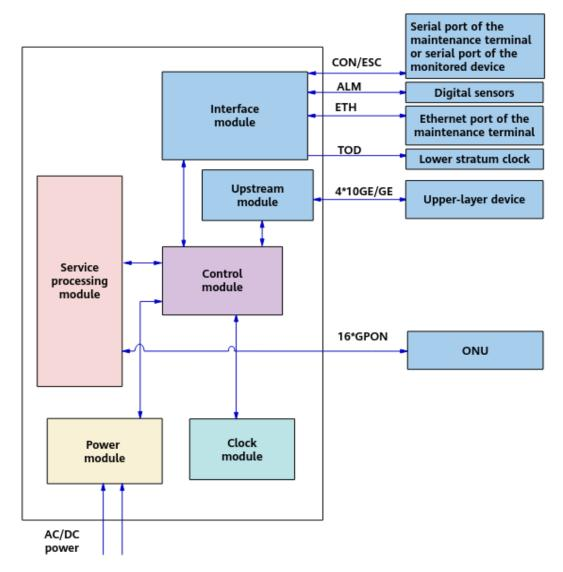
• **Control module**: It is the core of the system control and service switching and aggregation. It can also function as the management and control core of the integrated network management system (NMS).
