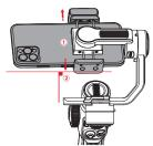
The balance state of the mobile phone will affect the gimbal runtime. The gimbal can work normally if unbalanced, but it will consume more battery power and weaken the motor strength.
