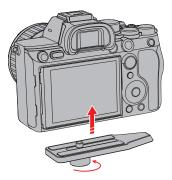
3. Toggle the quick release plate safety lock to unlock 0 , install the whole quick release plate on CRANE-M2 S 0 and make sure a firm installation.
