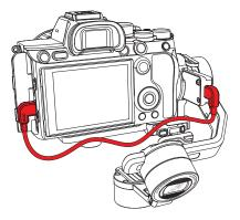
Q Please connect with the proper cable corresponding to the USB port type of the camera. For details of the compatible camera models, please visit the official website of ZHIYUN (www.zhiyun-tech.com) and check the "CRANE-M2 S Camera Compatibility List"
