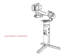
2. Mount the camera on the quick release plate. Tighten the screw.
