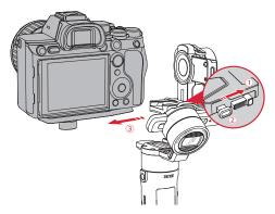
4. Connect the camera control port of the gimbal to the USB port of the camera.
