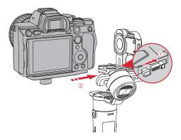
When detaching, toggle the quick release plate safety lock to unlock ①, press the quick release plate release button ② to push the whole quick release plate out ③.
