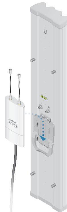
*The Rocket snaps into the built-in Rocket mount with ease.*
