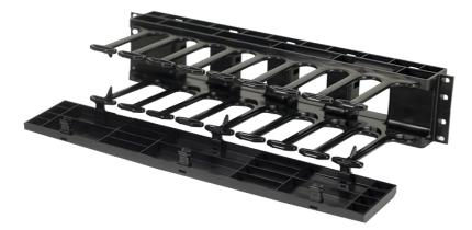
Horizontal cable managers are available in 1RU, 2RU, 3RU, and 4RU sizes. Fingers begin 3/4 in from the face of rack to provide bend limitation for cables, protecting cables, equipment and network performance. Included hinged cover mounts with six heavy duty clips allow them to be opened one handed without becoming "unhinged". Manufactured from UL94V-0 rated
