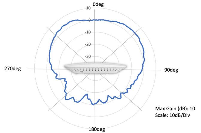
5 GHz Azimuth
