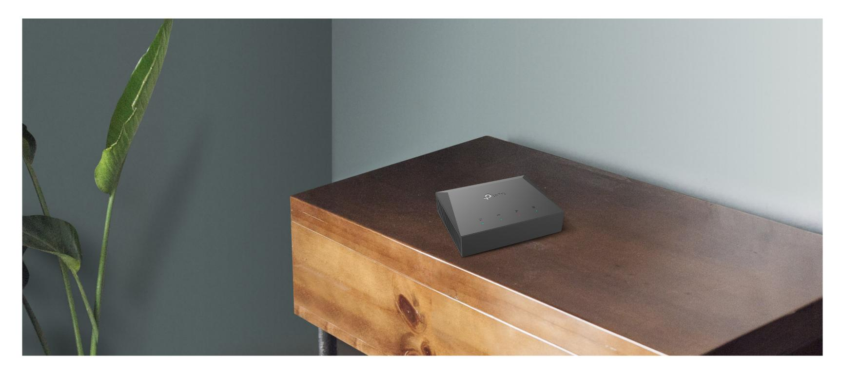
TP-LINK's XZ000-G3 is a next-generation Gigabit Passive Optical Network (GPON) terminal, ideal for Fiber to The Home solution. It's an incredibly robust device allowing users to access high-speed internet connections via its GPON port and share it with a Gigabit Ethernet port. With the transmission rates of up to 2.488Gbps, one GPON port and one Gigabit Ethernet port, the XZ000-G3 provides high-performance forwarding capabilities to ensure smooth VoIP, HD video streaming experiences.
